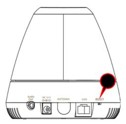
**Note:** Restoring the factory default setting will lose the all previous settings included IP address forever. User needs to run the IPWizard II program to search the device and configure it to let the device work properly again.
