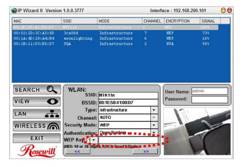
Double check your WLAN setting (Default using DHCP IP as your wireless router provides IP address for the Camera) then click "Submit".
