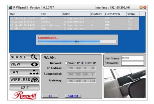
Once this step finished, IPWizard II will prompt you to unplug the Ethernet cable to activate wireless access. Then IPWizard II will prompt you to test wireless setting or finish wireless procedure as below.
