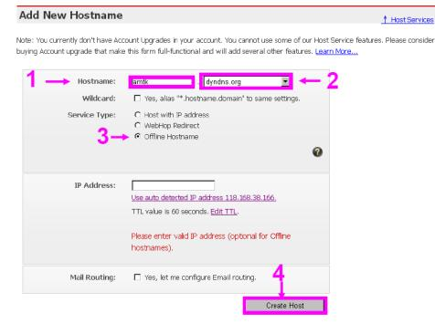
At last, you have to enter the web page of Networked Device and setup the necessary information of DDNS and PPPoE after the application of DDNS service. Please check the user manual to access the DDNS and PPPoE pages. After saving the modification, restart the device. Then the external users could browse the Networked Device by the input of their domain name.
