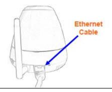
1. Please use cable connection for the first time setup. Using the RXS-4324 as example, please connect an Ethernet cable to the LAN socket located on the camera's rear and attach it to the network.
