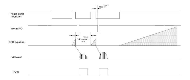
Note 1: The video output is going to be V reset by the next internal HD signal immediately after the exposure is finished. The exposure time is set by the pulse width of the trigger signal.
