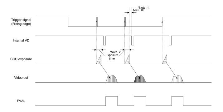
Note 1: The video output will be V reset by the next internal HD signal immediately after the exposure is finished.
