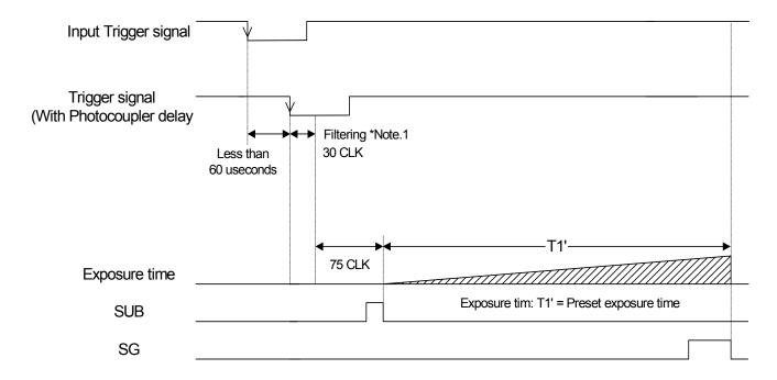
Note 1: The trigger signal will be removed by the filtering if the pulse width of the input trigger signal is less than 30 CLK.
