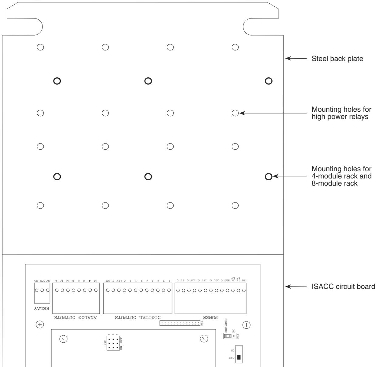
Pre-drilled holes in ISACC steel panel
