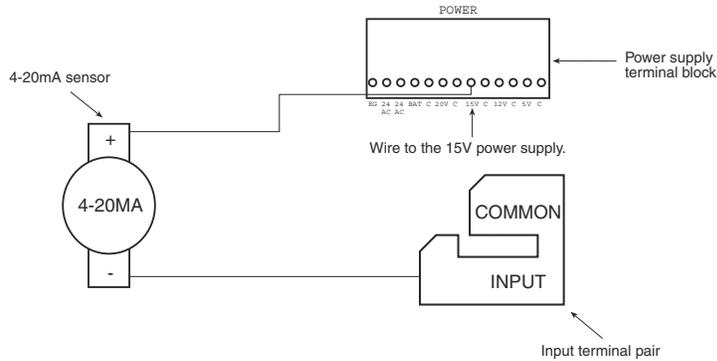
**4-20mA sensor using internal power supply**
