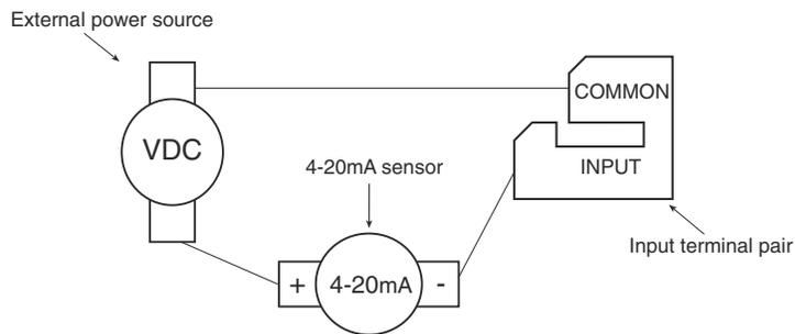
**4-20mA sensor using external power source**
