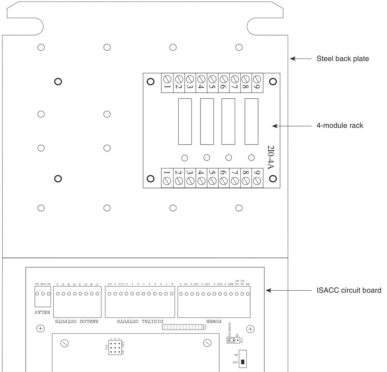
One 4-module rack mounted to steel panel
