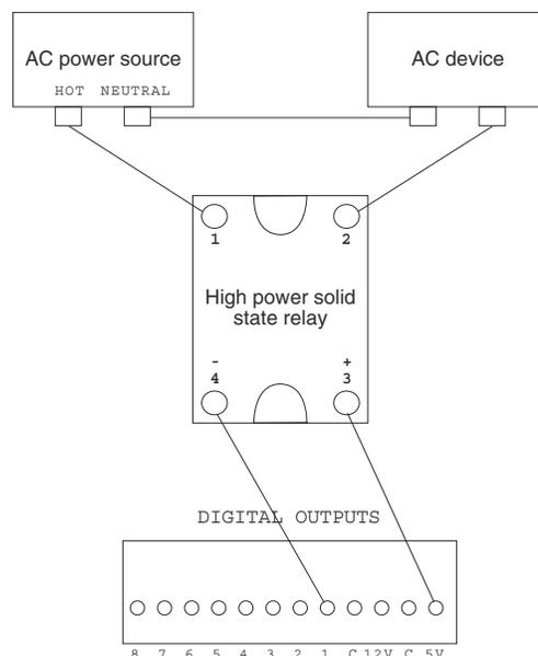
Wiring a high power solid state relay
