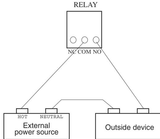
Wiring a device to mechanical relay using an external power source
