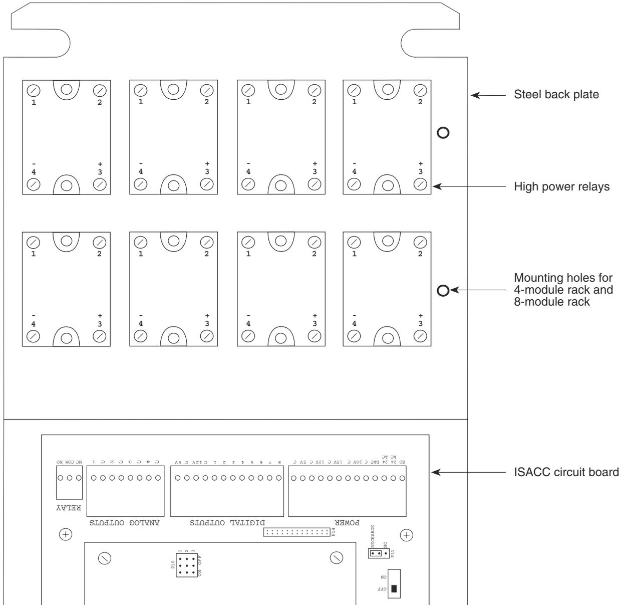
8 high power solid state relays mounted to steel panel
