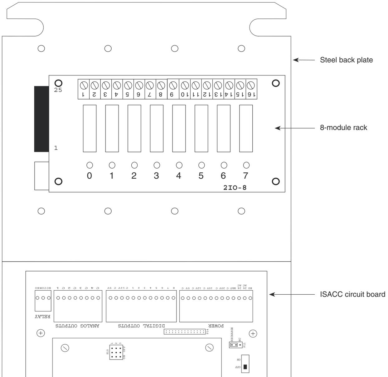
One 8-module rack mounted to steel panel
