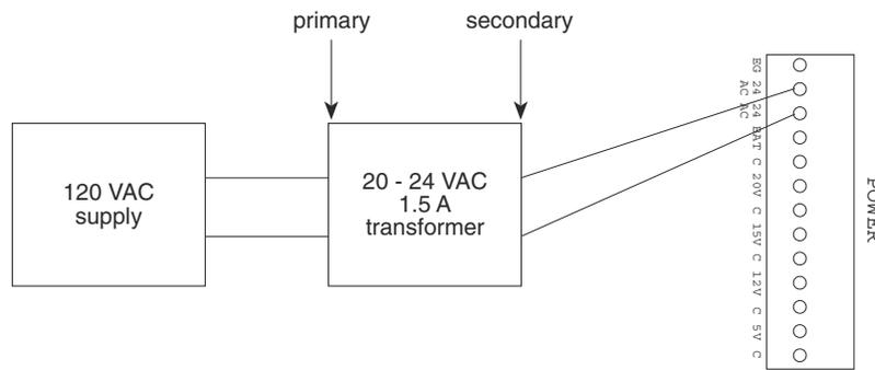
Wiring an AC power supply to ISACC
