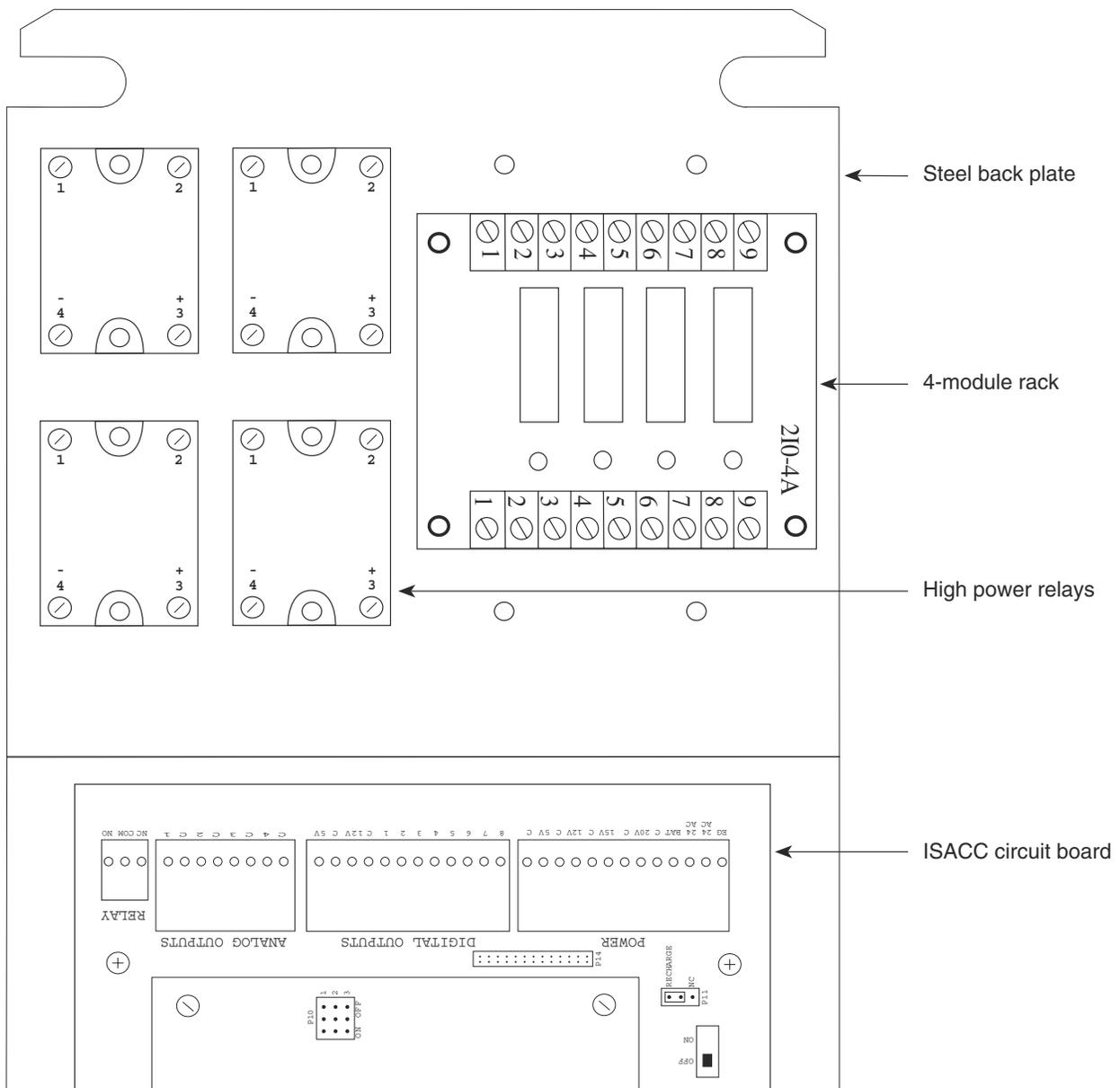
4 high power solid state relays and one 4-module rack mounted to steel panel
