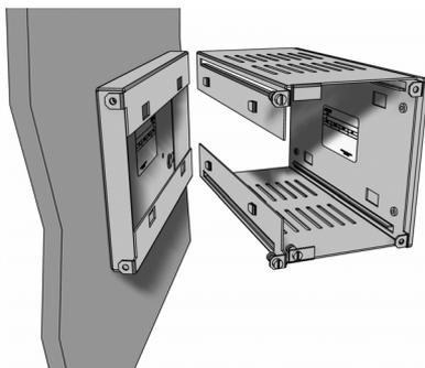
**Figure 2. Module Sleeve Attachment**
