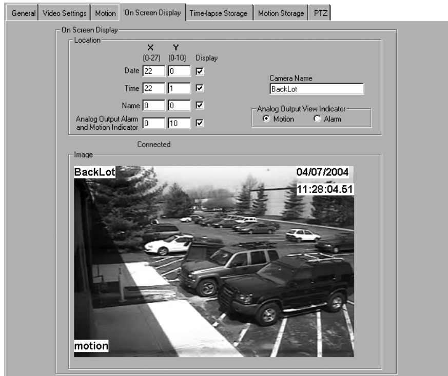
Figure 12. On Screen Display Tab for Configuring Video Text
