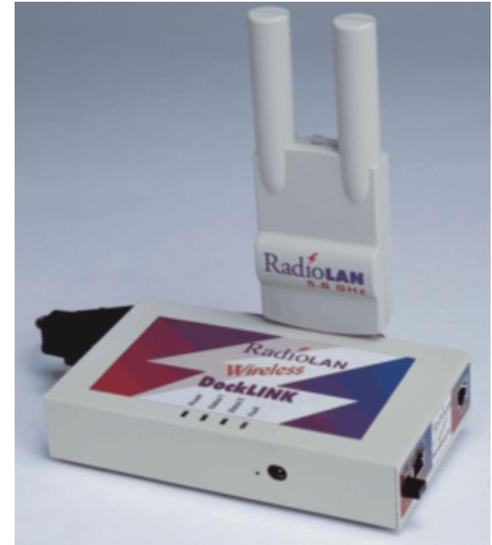
**Figure 1: The DockLINK and Radio Unit**
