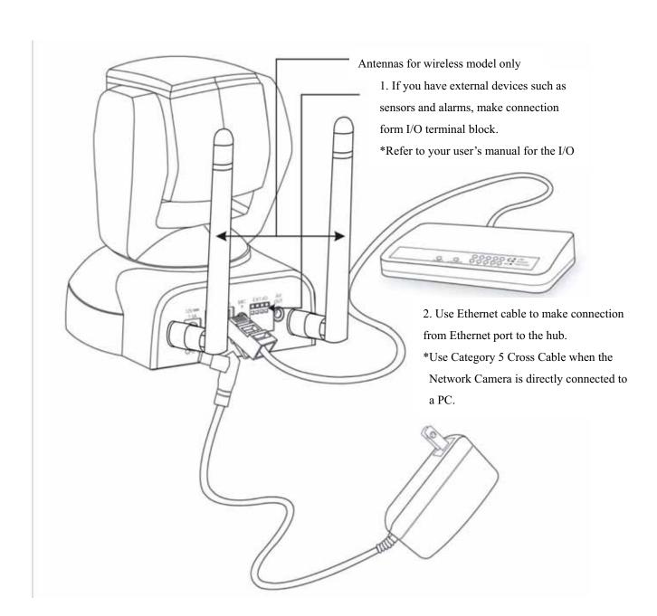
3. Finally, connect power cord to a power outlet.
