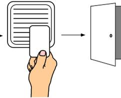
The relay activates for five seconds during which you must open the door. Once you open the door, you have 40 seconds to exit and close the door before the zone 2 Soft-Shunt expires.
