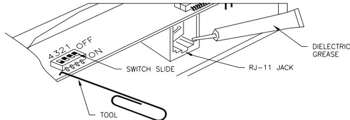
Coat reader connector with the silicone grease supplied to seal off moisture for outdoor mounting. To avoid having ESD (electrostatic discharge) interfering with the operation of the reader, the reader casing shall be grounded. This can be accomplished by tying the mounting bracket to earth ground locally (e.g. grounded conduit).
