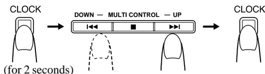
1. Press the CLOCK button on the Unit for more than two seconds.
