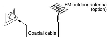
**Note:** Before attaching a 75 ohm coaxial lead (the kind with a round wire going to an outside antenna), disconnect the supplied FM Wire Antenna.
