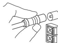
If reception is poor, connect the outside antenna.
