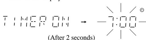
2. Press the ▶▶ or ◀◀ button on the Unit to set the time you want the Unit to come on.
