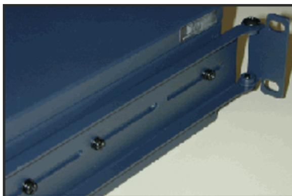
2. Rotate the hinges on both rails so that they allow the device to slide into the rack.
