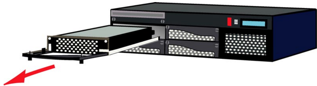
Fig. 42. Pull to remove a mounted hard disk from a unit; push to insert. Remove the front cover of the unit beforehand.
