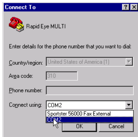
Fig. 19. Indicating a PC's COM Port, using HyperTerminal
