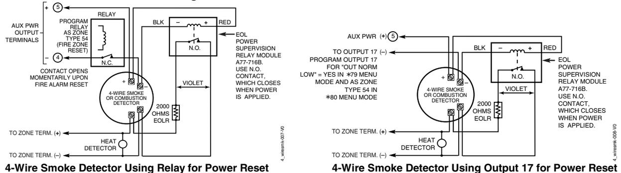
4-Wire Smoke Detector Using Relay for Power Reset
