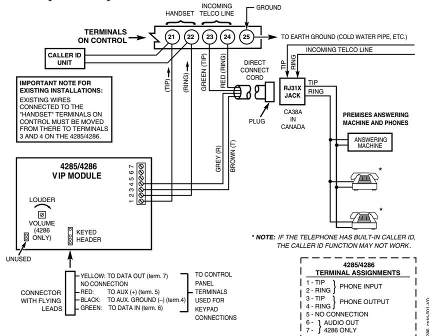
Figure 13. 4285/4286 Phone Module Wiring Connections
