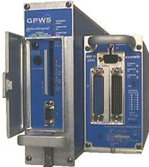
MK V & MK VII EGPWC (left) and MK VI, MK VIII, MK XXII EGPWC (right)
