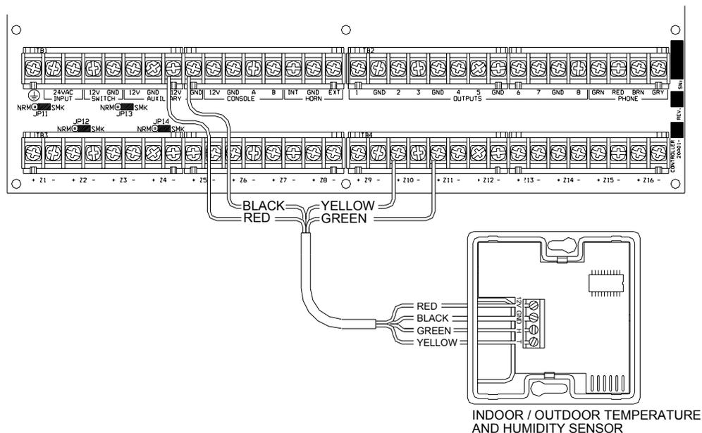
**FIGURE 11 - TEMPERATURE / HUMIDITY SENSOR CONNECTIONS**
