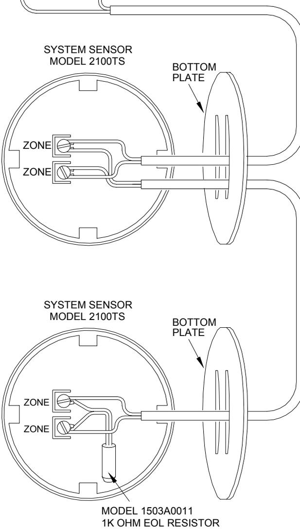
**FIGURE 3 - TWO-WIRE FIRE ZONE CONNECTIONS**
