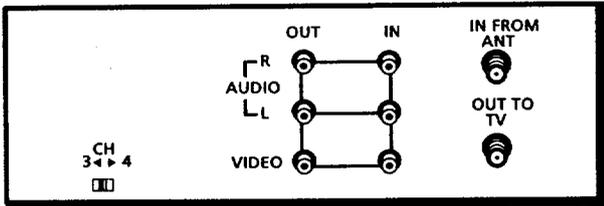
**3CH4 Switch** Selects the channel to which you will tune the TV to see the VCR picture if you connect the VCR using one of the basic hookups.
