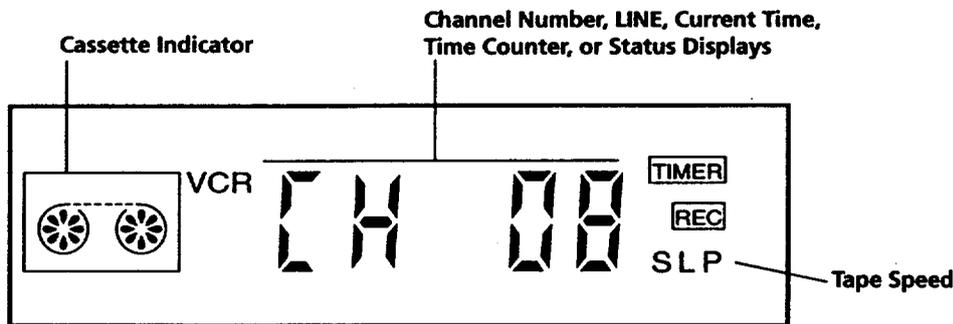
**Cassette Indicator** Shows when a cassette is inserted and displays direction tape is moving.
