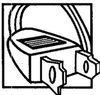
**Caution:** To reduce the risk of electric shock, match wide blade of plug to wide slot, fully insert.
