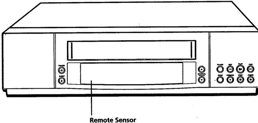
**CHANNEL•TRACKING Up or Down** Selects next higher or lower channel in the VCR's channel memory. Adjusts tracking when a tape is playing.
