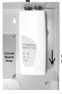
Slide Transceiver Over Mounting Plate to Secure it in Place
