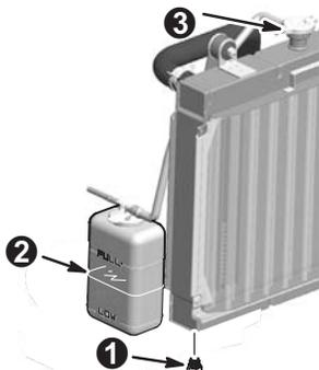
1. Remove drain plug ❶. As coolant is running out, open radiator cap ❷ to allow any trapped coolant to drain. Replace drain plug.
