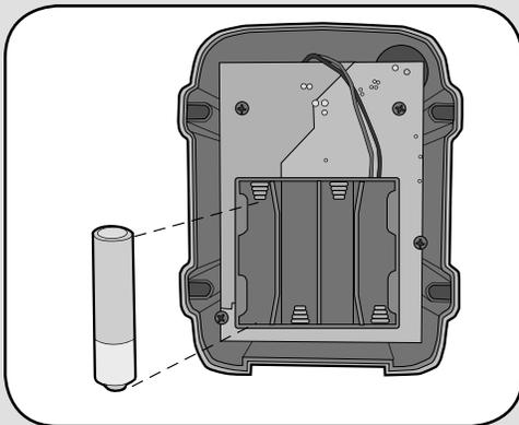
Install 4 AA Alkaline batteries (not provided). (Lithium batteries recommended for colder environments.) Keypad will beep. Keypad will continuously beep indicating no Master PIN Number has been programmed. Proceed to *Initial Setup*.
