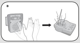
**B** Within 5 seconds, wave hand in front of PIR Motion Sensor. Test light will illuminate and Base Station will activate with static and feedback after several seconds.
