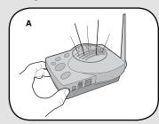
A Ensure that Base Station and PIR Motion Sensor are in close proximity to each other. Press and release learn button on Base Station. Buzzer will sound.
