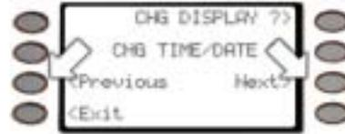
To exit the Command Menu, press the **<Exit** soft key.
