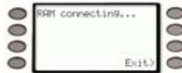
19. The security system will now call the telephone number or connect to the IP Address specified for network connection during the remote programming session.
