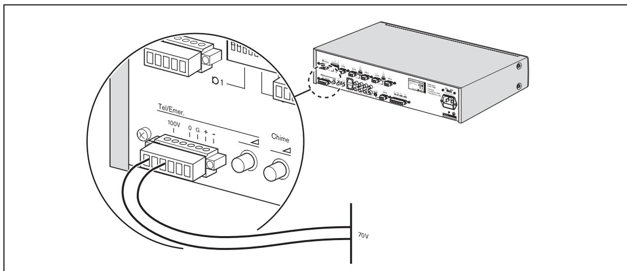
figure 4.4: Connecting 70 Volt input signal
