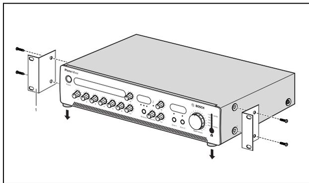
figure 3.1: Installing the unit in a rack
