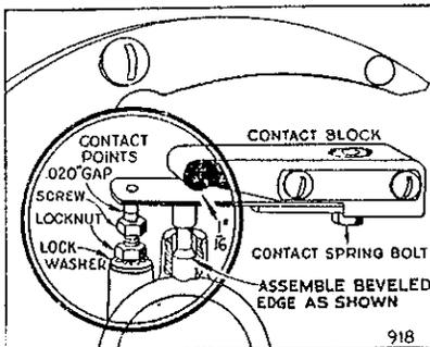
41. **TO REPLACE CONDENSER.** A leaky or weak condenser may cause the motor to start hard, to sputter, or misfire under load. If motor misfires after checking gasoline line, carburetor, spark plug, cable and contact points, install a new condenser. Slip the short insulator sleeve over the condenser wire. Solder the end of condenser wire and primary wire to contact spring. (See plate No. 13.)
