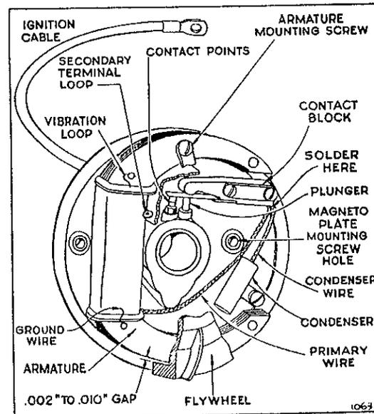
45. Air gap of .002" to .010" must be maintained between armature shoes and flywheel poles. Gap must only be sufficient to prevent rubbing but not over .010" or poor ignition will result.
