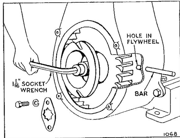
**36. TO REASSEMBLE THE FLYWHEEL** reverse the operations in preceding paragraphs, put a very thin coat of cup grease on the crankshaft taper and see that flywheel key is in place. Apply grease to starter gears.
