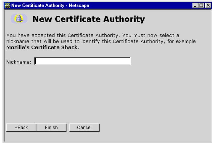
6. In the **Nickname** field, enter a descriptive name for this certificate. “Nickname” is something of a misnomer. We suggest you use a clearly descriptive name such as `Cisco VPN 3002 10.10.147.2`. This name appears in the list of installed certificates; see “Viewing Certificates with Netscape,” below.
