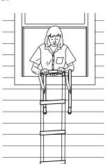
4. Exit carefully through the window and place your feet on the first rung. Hold onto the window frame until your weight is evenly distributed on the ladder. Climb down, keeping your body close to the ladder.
