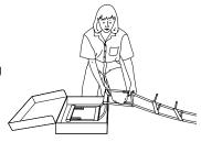
3. Use the plastic strap (attached to the last rung) to wrap and secure the rungs. This will minimize the chance of the ladder becoming tangled when you remove it from the box in an emergency.
