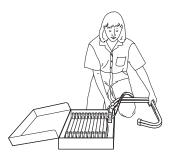
4. Lay the rungs, wrapped with the plastic wrap, in the box with the standoffs facing upward. Place the folded sill hooks on top of the rungs, between the standoffs.
