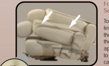
Folding the Outboard Seats to a Full-Lowered Floor Position
