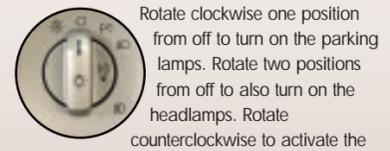
Rotate clockwise one position from off to turn on the parking lamps. Rotate two positions from off to also turn on the headlamps. Rotate counterclockwise to activate the autolamp, which provides light-sensitive automatic on-off control of the exterior lights and keeps them on for a short period of time after the ignition is turned OFF. When the control is in any position except high beams or off, pull the control toward you to activate the foglamps.
