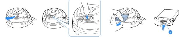
➤ Connect the charging cable ② to the socket for charging cable ③ on the battery pack.
