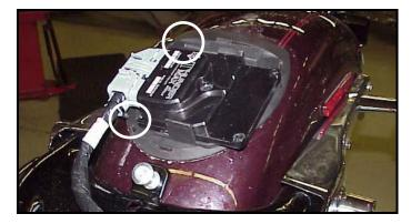
**Step 2c** Install the AutoTune module. Mount the AutoTune module to the frame backbone using supplied wire ties (right side view below). Position housing so wires exit to the left as shown below.
