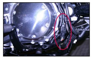
**Step 2g** Rear sensor: Route wiring down the left frame rail behind the primary housing, with the plug located along the frame turn. Double-back the wiring to the rear sensor. Connect the sensor to the closed loop module, secure with wire ties.
