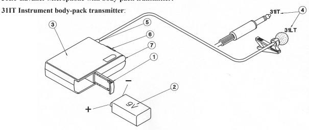
(1) Open the battery compartment lid by sliding it down and raising it.
