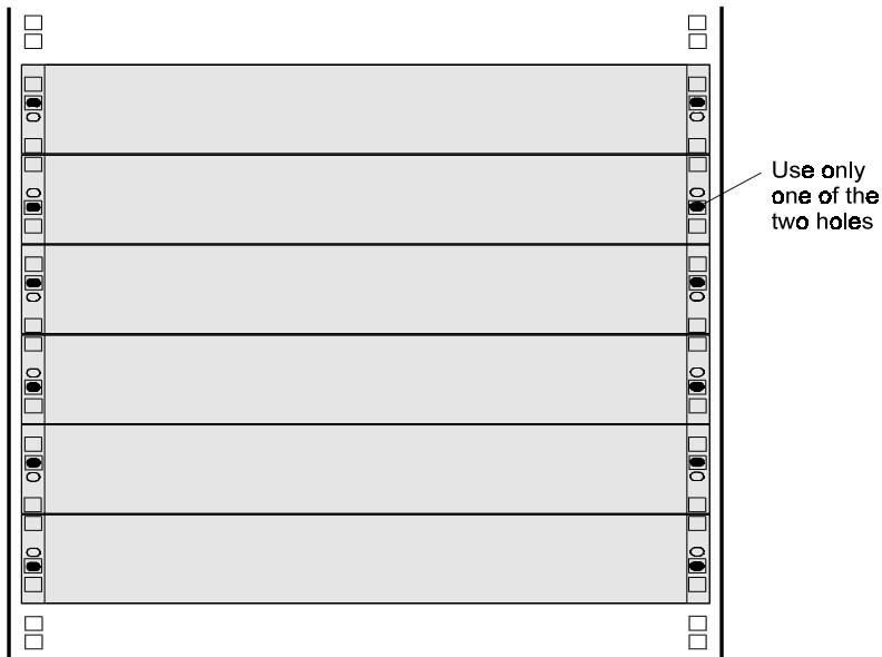
Figure 3 Cajun rack mounting arrangement
