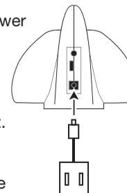
When the adapter is inserted into the base unit and plugged into a wall socket, a red light on the front of the base unit will light up to indicate that power is active.
