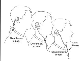
Tighten the cable and take up slack by raising the cable sleeve.
