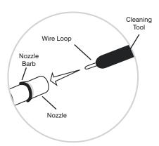
When cleaning, do not force any object through the earphone nozzle! This will damage the earphone sound filter.
