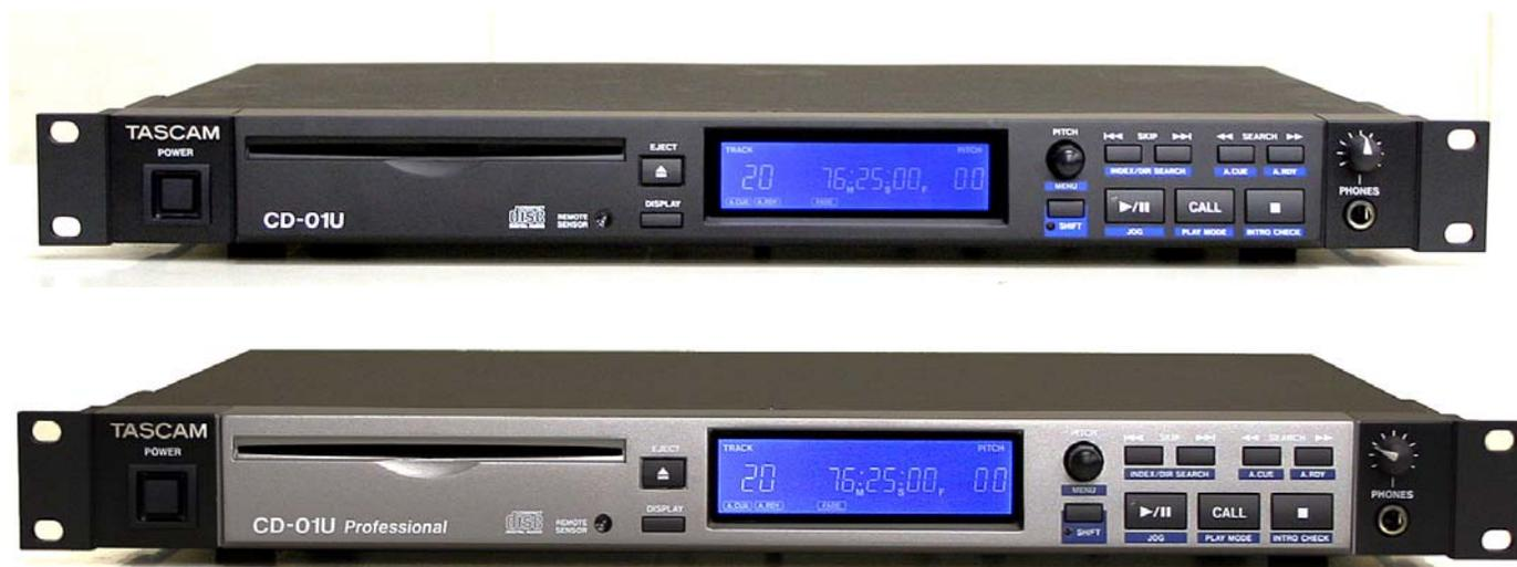
The CD-01U / CD-01UPRO are 1U rack mountable CD players with **slot loading** transports. The CD players provide multiple playback modes, auto cueing, auto-ready, Intro-Check, Pitch Control (+/- 12%), Key Original Function, and fade in/out function ( up to 10 seconds in ½ step increments). The CD players are equipped with 20 seconds of RAM buffer for shock protection and both are RS-232 controllable.
