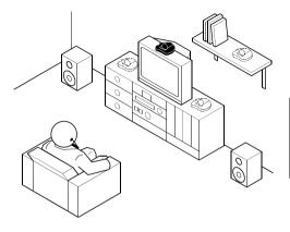
If there is no audio signal for about 3 minutes, the transmitter automatically turns off. The transmitter is now in stand-by mode, its power consumption is very low so that it can remain connected to the mains. Batteries can always be recharged when the transmitter is connected to the mains.
