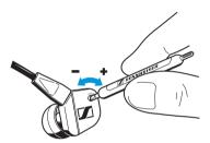
➤ To increase (+) or reduce (-) the bass response, turn the control using the supplied adjustment tool.
