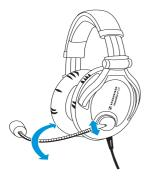
Bend the microphone boom 3 so that the microphone is placed at the corner of the mouth. Maintain a distance of approx. 2 cm between microphone and mouth.
