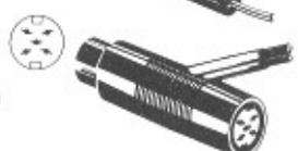
The "DIN headphone multiplug" is built in a way to allow connection of further headphones. It has to be considered, however, that all headphones joined in this way are connected in parallel, therefore total impedance is divided by the number of units connected. It has to be checked whether the sound source is suitable for this kind of loading.
