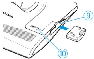
When the battery is inserted correctly, the indicator ⑩ lights up:
