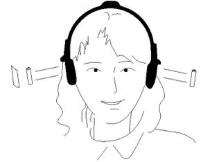
When using the AAANi-Cd Rechargeable battery in your headphones, you must charge for 24 Hours prior to first use.
