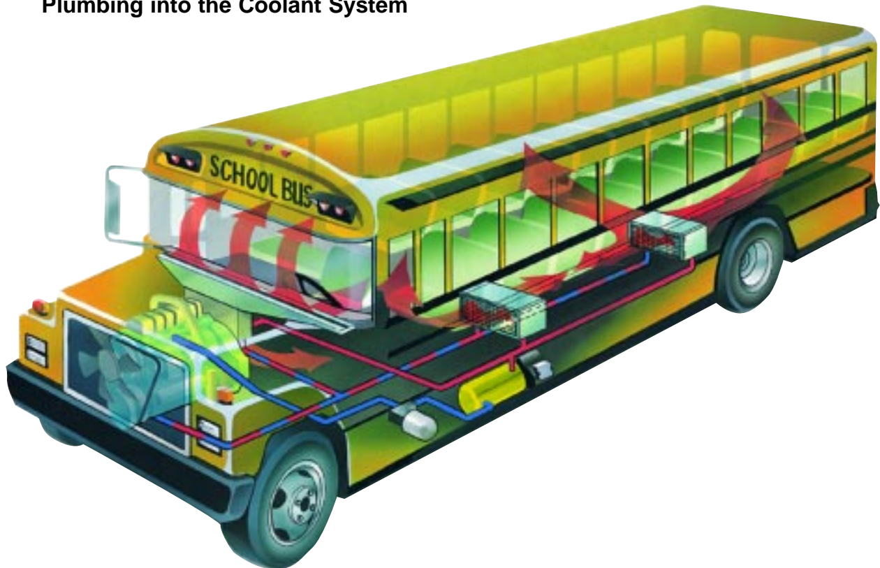
Fig. 5-3: Typical School Bus Heating Circuit
