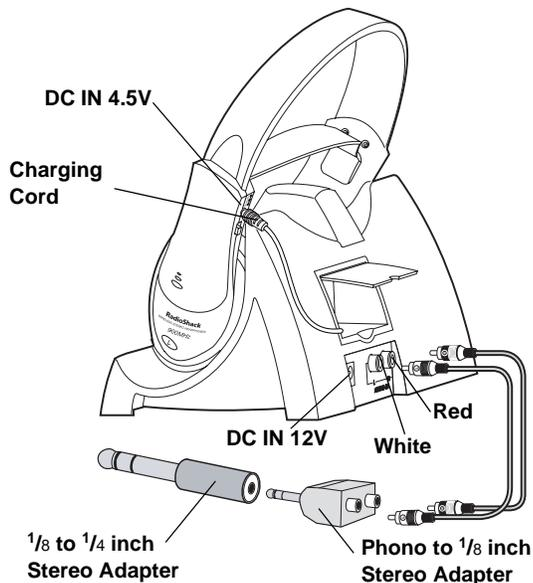
6. Plug the charging barrel plug into the **DC IN 4.5V** jack on the left earpiece.
