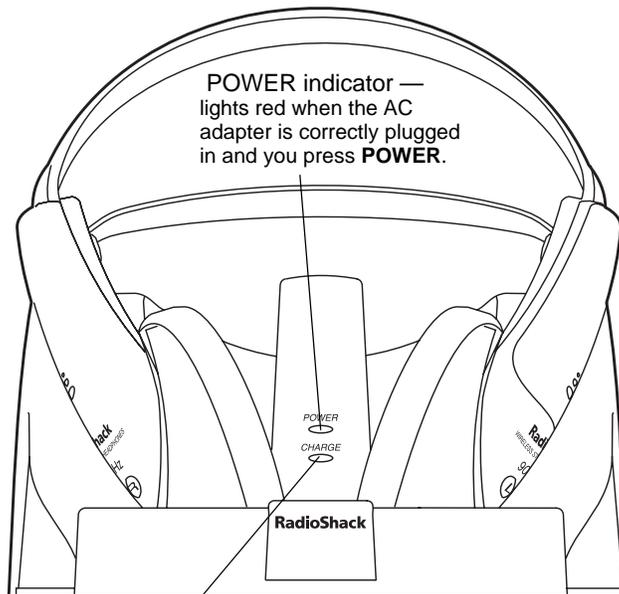
POWER indicator — lights red when the AC adapter is correctly plugged in and you press **POWER**.
