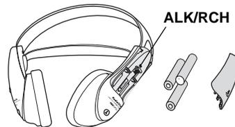
2. *If you are using alkaline batteries*, set **ALK/RCH** inside the compartment to **ALK**.
