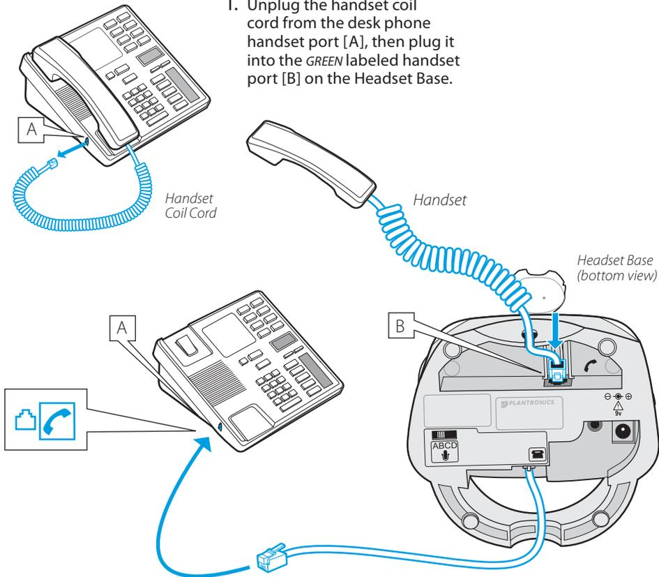
2. Plug the short **BLACK** Phone Cable that is pre-installed on the Headset Base into the now-open handset port [A] on the desk phone.
