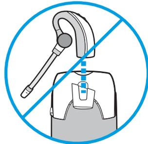
**IMPORTANT!** Make sure the headset is facing correctly (as shown at left) when inserted into the charging cradle.
