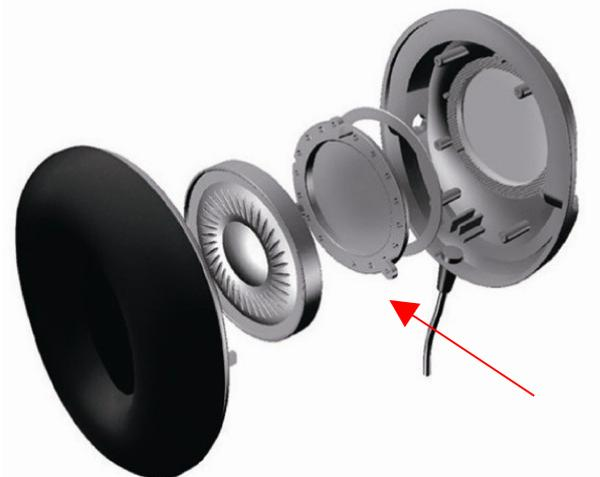
Ring Port Structure provides high-quality dynamic sound. With a ring port structures sound ports located in a circle behind the driver unit, the sound pressure in headphone housing is equalized, realizing stable amplification in the unit as a whole.
