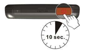
NOTE: For normal operation, briefly press the power button to turn on and off your device.
