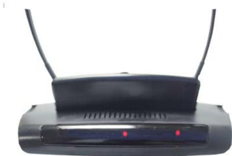
**figure 3** 2 LED's show the unit is charging.
