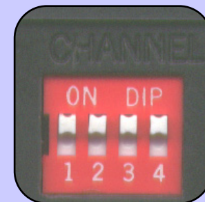
EASY TO CHANGE CHANNELS WITH 4 DIP SWITCHES
