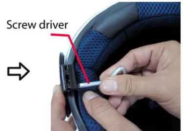
**Note:** If the helmet's shell is too thick, the **Spacer** (provided) may be needed to put in between the 2 parts of the Headset Clip, as shown in the picture on the right. Use the additional longer screws (provided) for this purpose.
