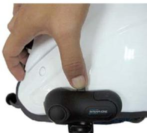
Remove the BlueAnt InterPhone by pushing down the lock as shown and then take out the InterPhone Module in an upward motion.
