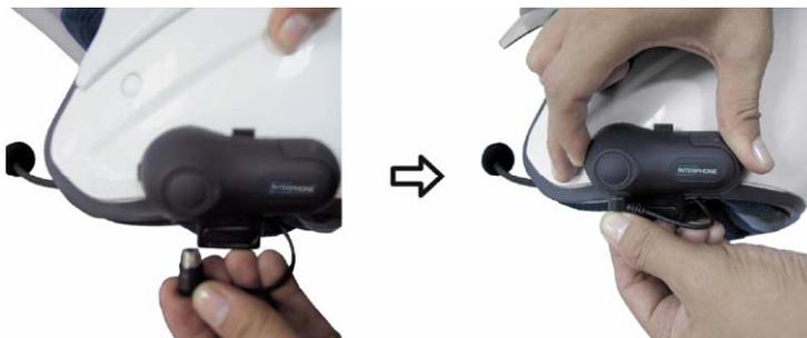
5. Secure the cord of the **Headset Plug(9)** inside the helmet. Tuck any extra wire into the helmet. Ensure that only few centimeters of the cord comes out.
