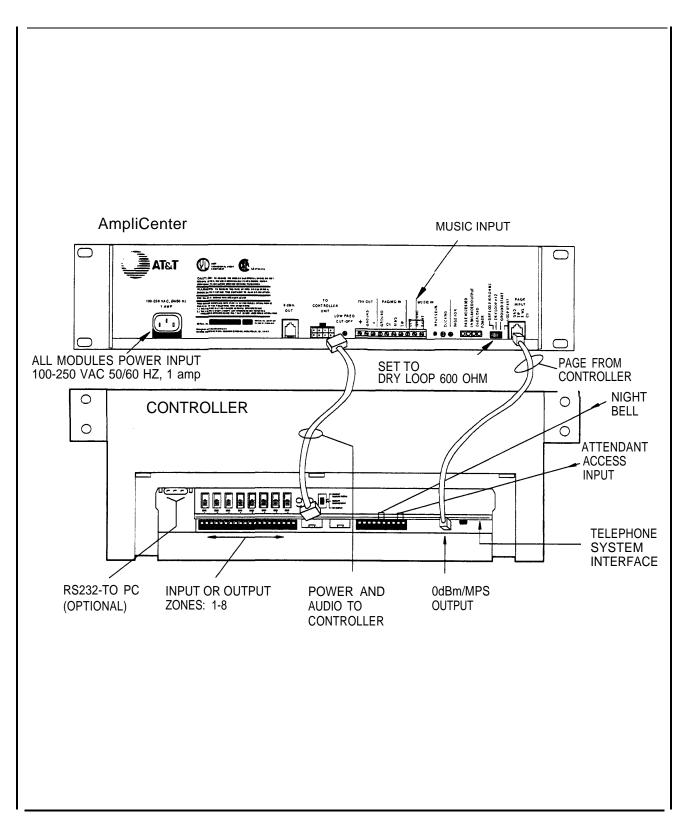
Figure 3-1. AmpliCenter Interface with PagePac Plus Controller
