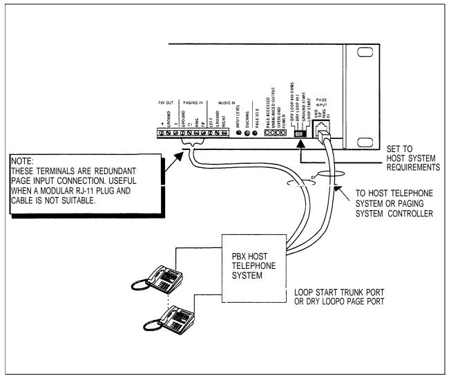
Figure 3-6. AmpliCenter Interconnection to Telephone System or to Controller
