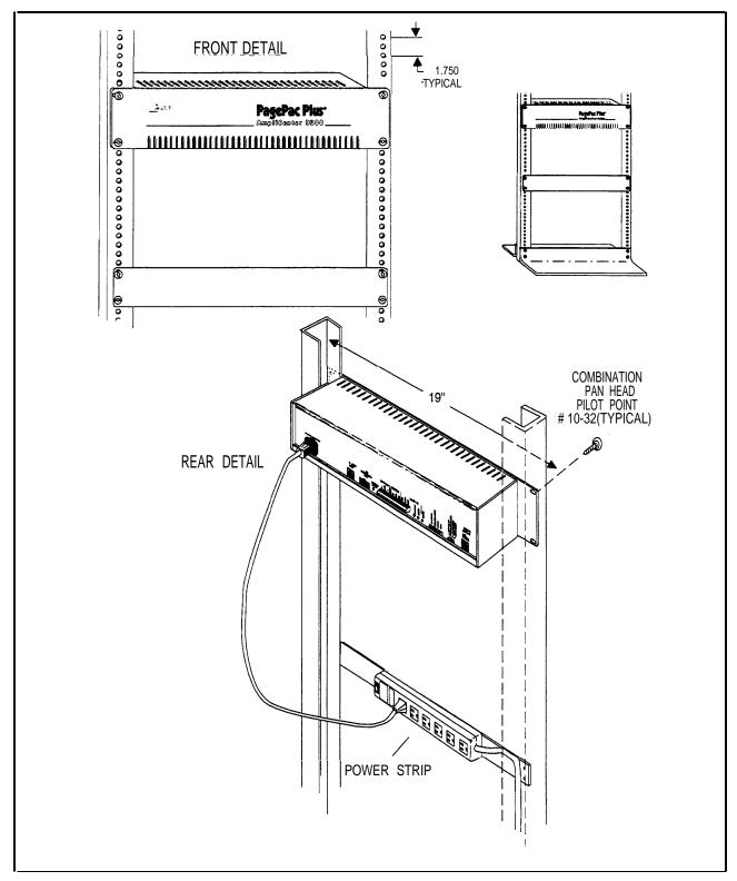
Figure 3-4. Rack Mounted Hardware
