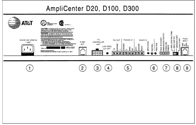
Figure 2-1. AmpliCenter Controls and Indicators, Terminals and Connectors
