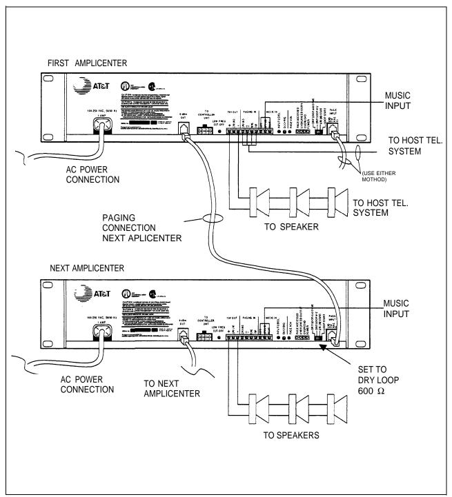
Figure 3-2. Series AmpliCenters, without Controller
