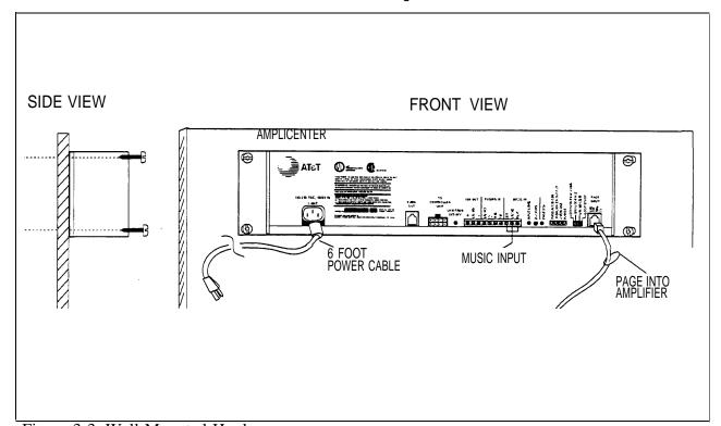
Figure 3-3. Wall Mounted Hardware
