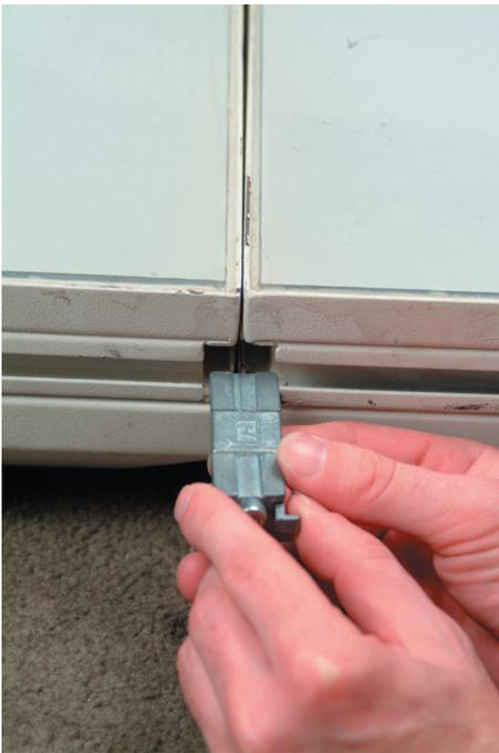
1. Put two dance floors side by side. Take the Dance floor connector (Part# SCA-5) and loosen the allen wrench thumb screw, turn it sideways and start sliding between the two dance floors. If it is difficult to slide in, loosen the thumb screw a little more.
