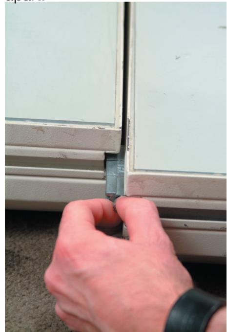
5. With the two dance floors separated reach in and grab the connector and slide it out.
